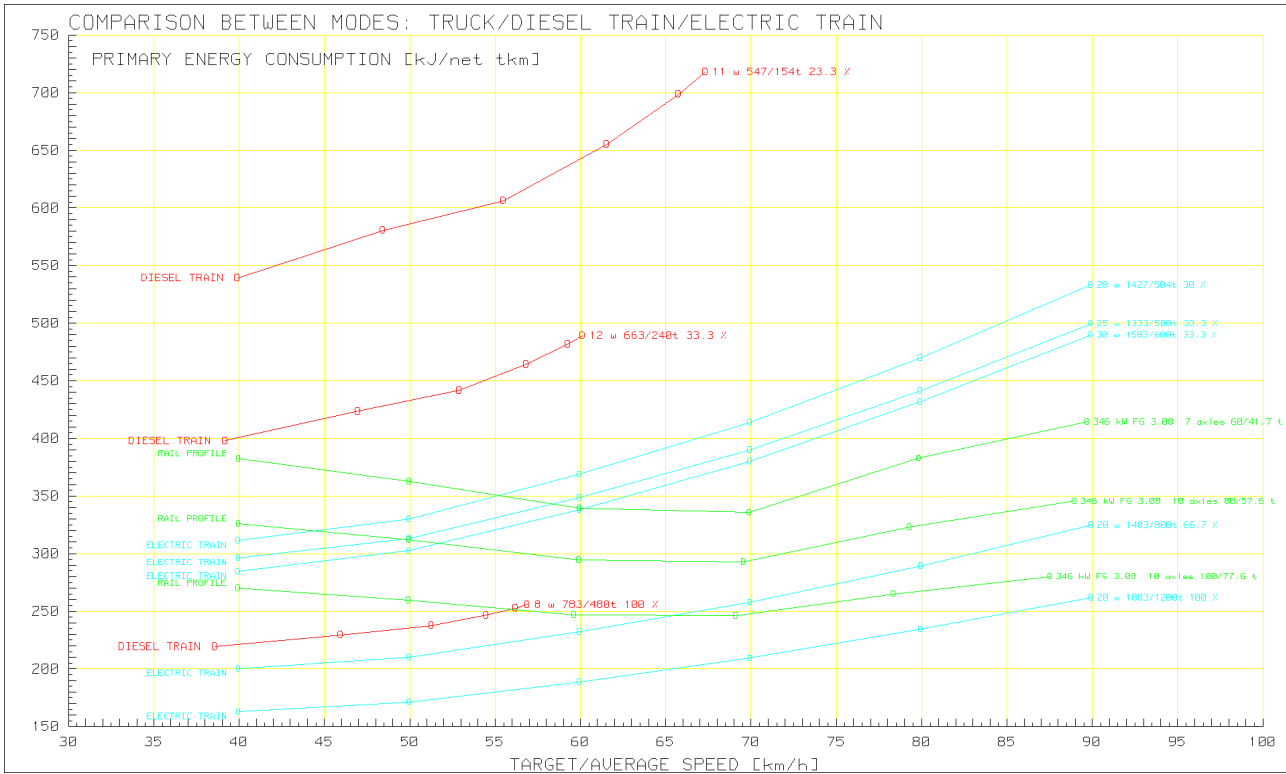
Fig. 7B Comparison between truck and trains. Truck route is rail profile
